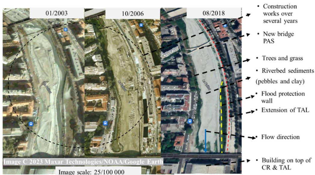
Figure 43 Impacts of construction works on land-use in of LPR bed in Nice urban centre 2003 to 2018 (Google Earth Images).
