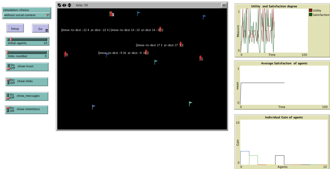
FIGURE 3.5: The user interface of our Multi-Agent simulation environment in Netlogo. The person icon represents an agent in the MAS. Flags represent destinations in which agents can go. Labels represent agent intentions which consist of two elements: the name, mapped to a NetLogo command, and a done-condition, mapped to a NetLogo reporter. Intentions are stored in a stack, and are popped out when to be executed. If the done-condition is satisfied, the intention is removed and the next intention is popped out consecutively. The Figure shows also, on the right-hand side, how the graphs are updated dynamically as the program runs.
