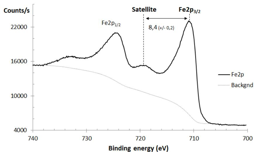
**Fig. 4** Fe2p XPS spectra of magnetic biochar
