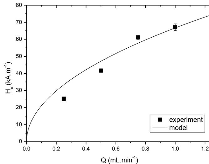
**Fig. 11** Critical magnetic field ( $H_c$ ) as a function of flow rate ( $Q$ ): experimental data and modelling
