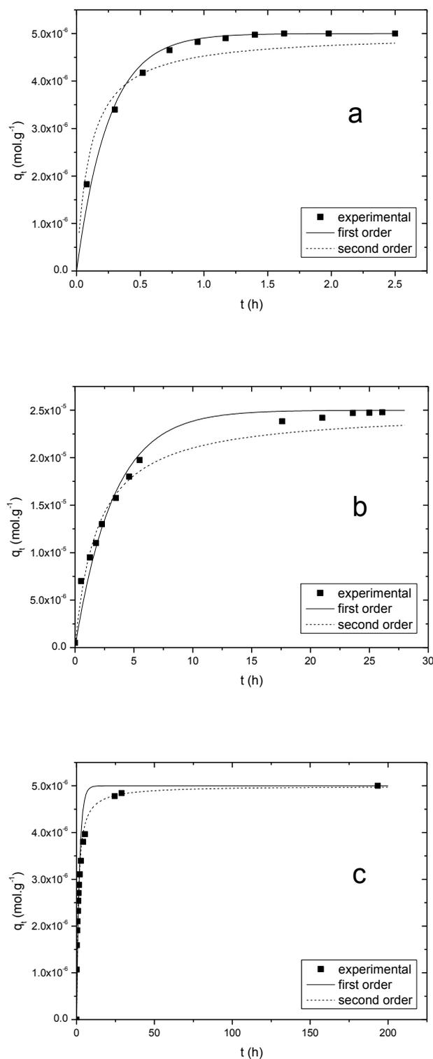
**Fig. 9** Kinetic data and modeling of the adsorption of methylene blue onto magnetic biochar (a:  $C_0 = 2 \cdot 10^{-5}$  mol.L<sup>-1</sup>; pH = 6 / b:  $C_0 = 10^{-4}$  mol.L<sup>-1</sup>; pH = 6 / c:  $C_0 = 2 \cdot 10^{-5}$  mol.L<sup>-1</sup>; pH = 2)
