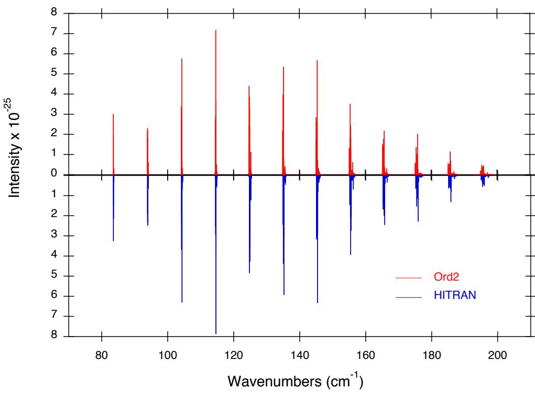
Fig. 2. Calculated R(7-18)-spectra versus spectra from HITRAN database (upside-down). 388 transition lines are present in both spectra corresponding to an intensity cutoff of  $10^{-32}$   $\text{cm}^{-1} / (\text{molecule.cm}^{-2})$ .
