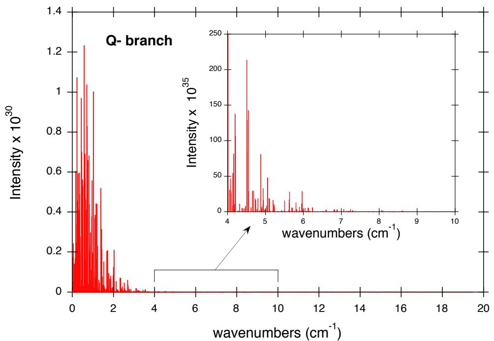
Fig. 4. *Ab initio* Q-Branch spectra for  $J \in \{1, 30\}$  corresponding to the transition wave numbers and intensities given in supplementary material.
