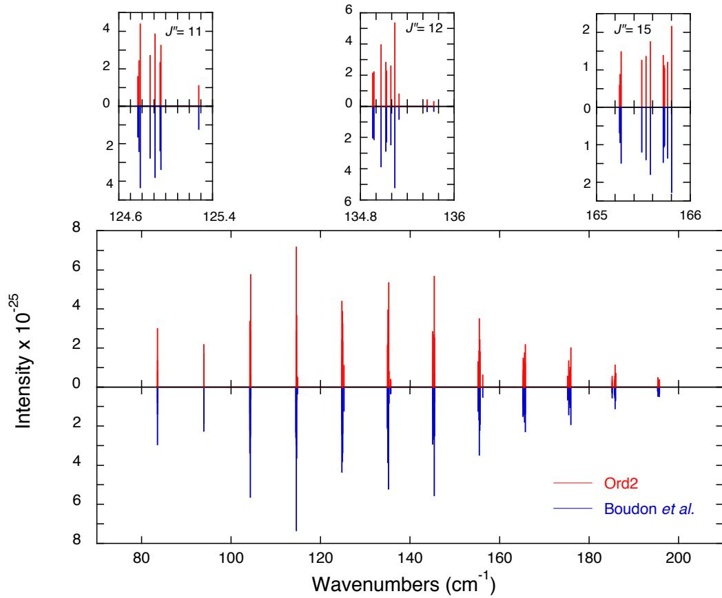
Fig. 1. Calculated R(7-18)-spectra versus observed spectra (upside-down). 93 transition lines are present in both spectra. The three panels above the main panel represent enlarged regions corresponding to a given lower level  $J$ -value.
