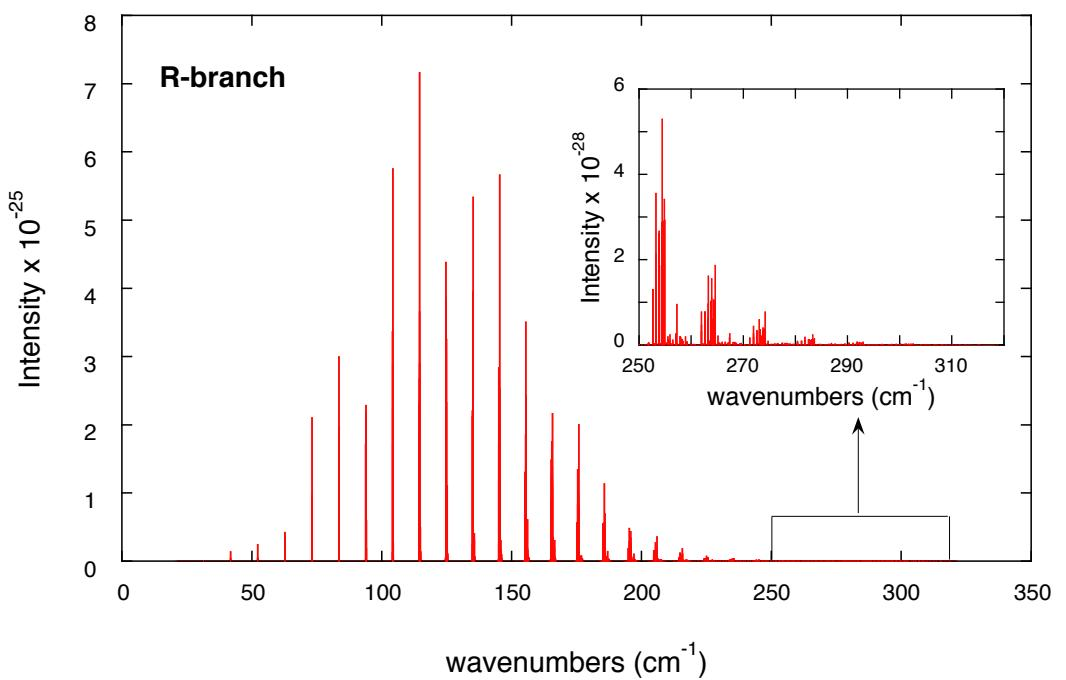
Fig. 5. *Ab initio* R-Branch spectra for  $J \in \{1, 30\}$  corresponding to the transition wave numbers and intensities given in supplementary material.
